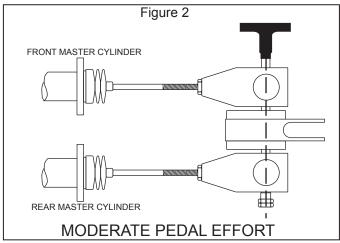
Please note: the above pushrod adjustment is for a typical dirt application with small front calipers and large rear calipers.
